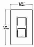
BluetoothVersion:4.2 Housing Material: UL 94-VO Indoor Use Only Operating Temperature: -18°C to 50°C, -0.4°F to 122°F Storage Temperature: 0°C to 30°C, 32°F to 86°F IP Rating: IP20 Color: White Warranty: 5 years warranty
