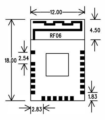
Note: When using onboard antenna, please keep the antenna at least 15mm away from other metal components. No wire or copper around the antenna.
